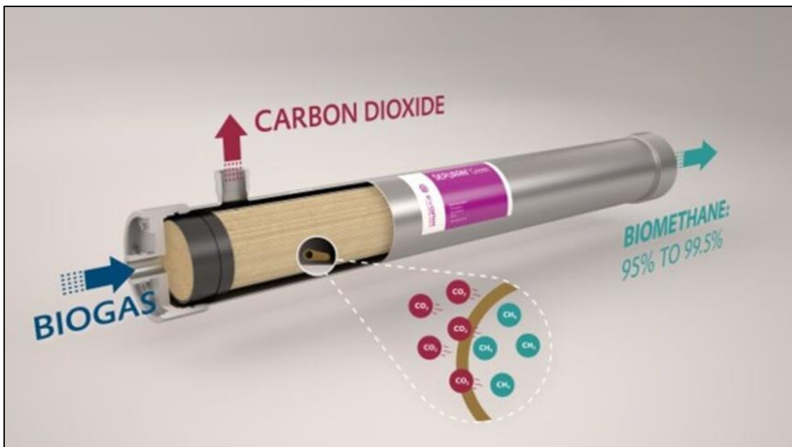
Figure 12: Upgrading of biogas to biomethane with membrane module (Example: EVONIK SEPURAN® Green membranes)
