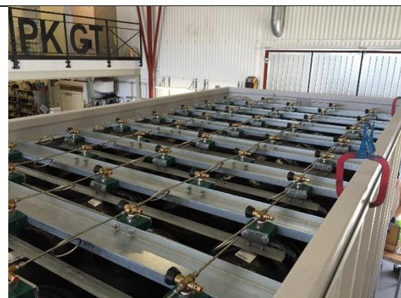
Skid with composite cylinders under production
