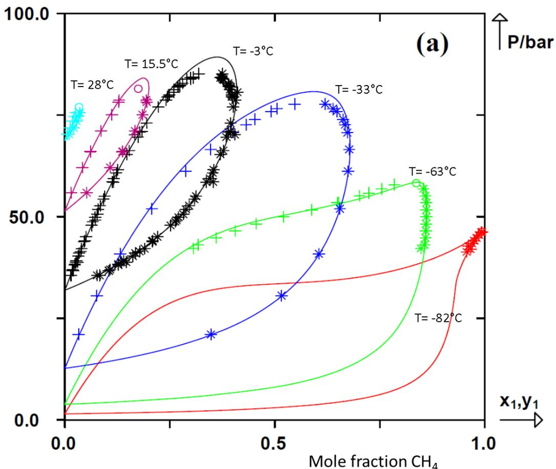
Figure 7 At temperatures above -33 C, liquid CO<sub>2</sub> will not form if the CO<sub>2</sub> concentration is below approximately 32%, and thus CH<sub>4</sub> higher than 68 % (from Privat and Jaubert <sup>5</sup>).
