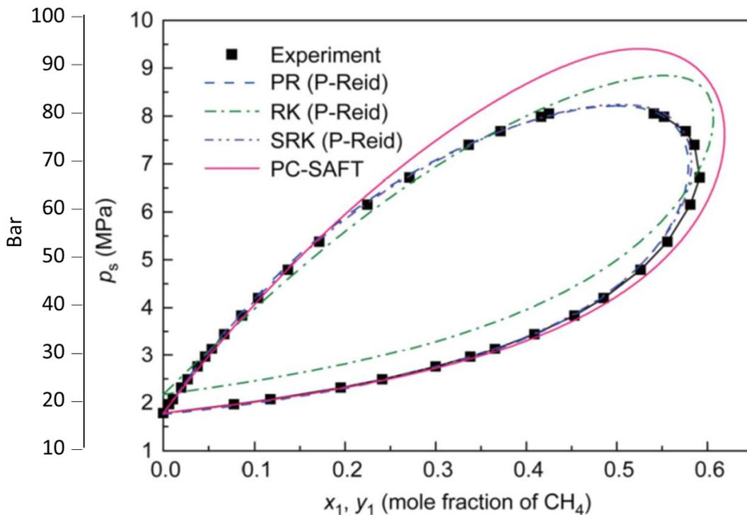
Figure 6 Mole fraction of CH<sub>4</sub> in both phases calculated by different Equation of States models compared with experiment (modified from Yang<sup>4</sup> et al.)
